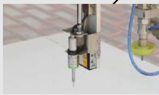
Laser height measurement & probe detection 激光测高&探针探测
