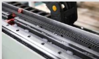
Oil-immersed linear guide rail 油浸式直线导轨
