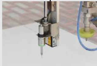
Laser Height Measurement & Probe Detection 激光测高 & 探针探测
